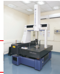
Coordinate Measuring Machine (CMM), MITUTOYO, CRYSTA-Apex S7106 Measuring Range 700 X 1000 X 600 mm, Resolution 0.1 µm, Software – MCOSMOS-III (CNC)
