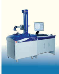
Roundness Measuring Machine, Taylor Hobson, Talyround 565LT Column height = 500 mm, Max Loading Diameter = 485 mm Max Diameter of Measurement = 435 mm Rotation Accuracy = +/- (0.015 µm + 0.0003 µm / mm) Straightness Accuracy = 0.25 µm over 200 mm Parallelism Accuracy = 1 µm over 500 mm Max Load Capacity = 75 Kgs
